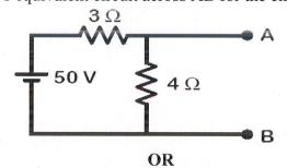
4 Find the Short circuit parameters for the given circuit.
